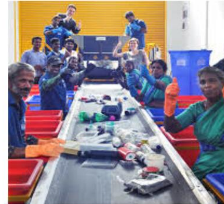
Platform for secondary segregation of dry waste
